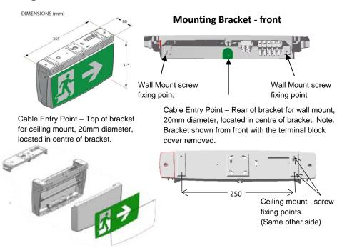
**Changing Exit Legend Inserts:** The Cleverfit Exit uses Clevertronics patented "Tamper proof" Exit legend cover and comes complete with spare legend inserts to enable straight on, left or right arrow as well as SS/DS combinations.
